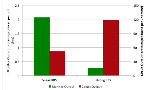
Fig. 5. Modelled impact of RBS strength on circuit and monitor output in the fast codon case. These simulation data show that a stronger RBS causes higher circuit output and lower monitor output.
