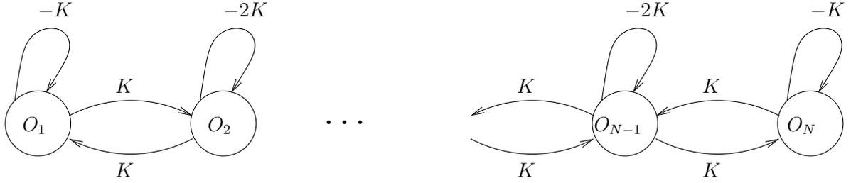
Figure 4.10: Synchronizing bidirectional open chain structure.
