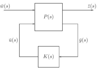
Linear Fractional Transformations (LFT's) are a useful way of manipulating closed-loop transfer functions, and of specifying norm-optimal control problems. The lower LFT  $\mathcal{F}_l(P(s), K(s))$  is defined as the closed loop transfer function from  $\bar{w}(s)$  to  $\bar{z}(s)$  in the above picture. That is
