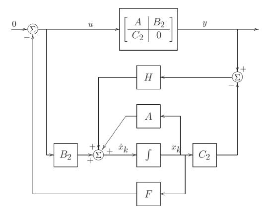
$\label{eq:closed-loop poles of optimal } K = \lambda_i \underbrace{(A-B_2F)}_{\text{stable}} \cup \lambda_i \underbrace{(A-HC_2)}_{\text{stable}}.$
